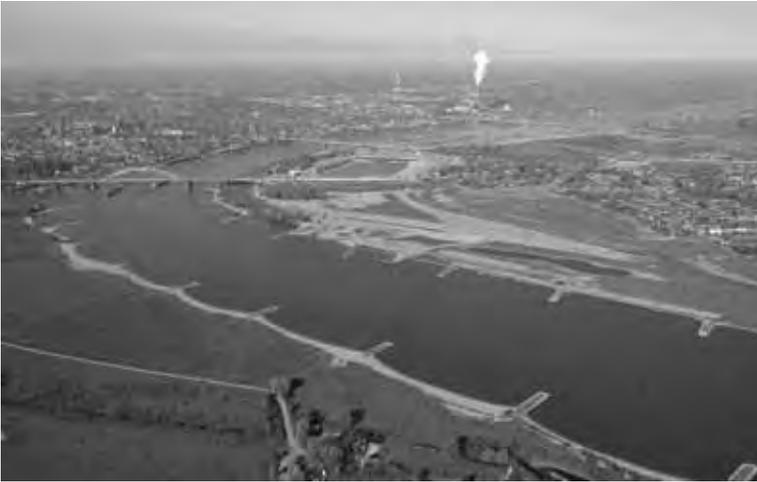
*Figure 10. New channel and formation of island in the River Waal
