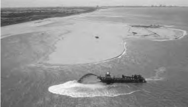
*Figure 3. Sand dredging the Sand Motor*
